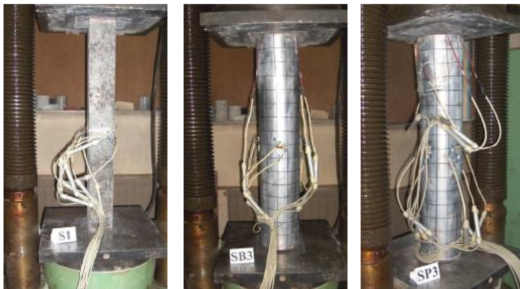
Slika 7. Modeli ispitivanih stubova a) kontrolni uzorak, b) ispuna sitnozrni beton, c) ispuna Polimag HK-08 Figure 7. Tested column samples: a) control sample, b) sample filled with concrete, c) sample filled with Polimag HK-08
